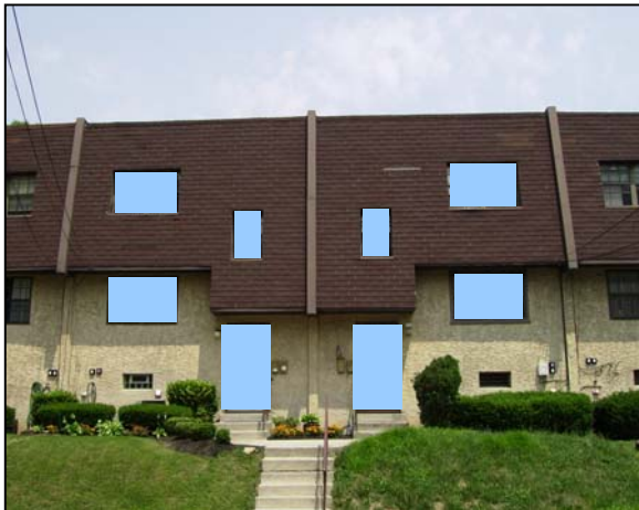
This building has a wall to opening ratio of approximately 5 to 1 and is not compatible with Lansdowne's traditional buildings.
